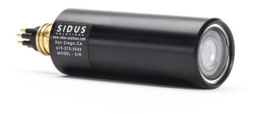
SIDUS Solutions' SS408 is a lightweight, durable and compact black and white camera. It is one of our smaller miniature cameras available. Designed for high sensitivity in low light, this camera employs a 1000 TVL color module that has a 1/3" 2MP Panasonic CMS imaging sensor capable of sensing light as dim as 0.008Lux and 0.0008Lux with sensup.
